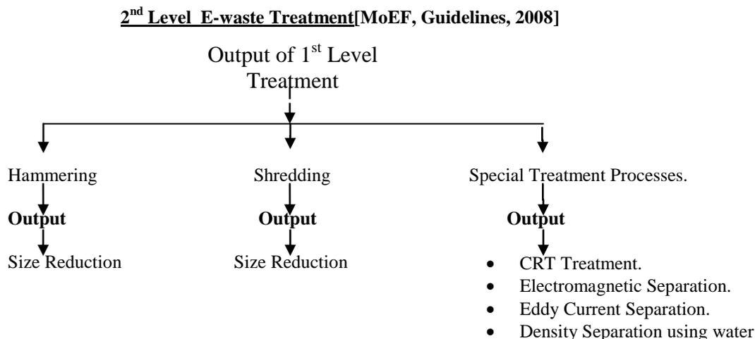
Fig: 10 Flow chart of 2<sup>nd</sup> level e-waste treatment.
