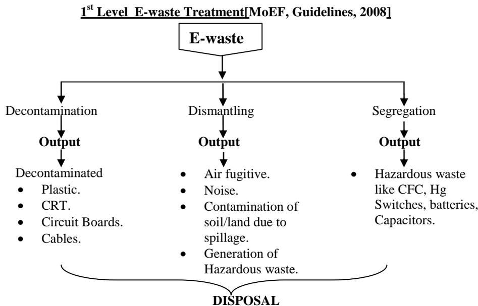
Fig. 9 Flow Chart 1<sup>st</sup> Level Treatment
